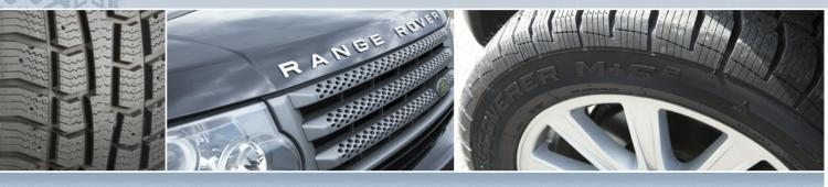
**Directional Tread:** Modern directional tread for improved traction with low noise levels, featuring tread blocks with Lamellen siping improving traction and braking in the most severe winter conditions of snow and ice.
